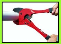
Two hand operated ratchet cutter that cuts all types of PVC (thin wall, Schedule 40, and Schedule 80), CPVC, ABS, PE, polypropylene (PP-R) and PEX pipe and tubing through 2-1/2" (63.5 mm) nominal pipe size.
