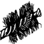
**A POOR QUALITY FITTING BRUSH** is a brush that has ragged and uneven bristles and is less effective.
