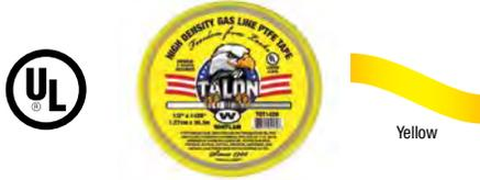
**TALON YELLOW GAS LINE PTFE TAPE** 3.5 Mil Thick, 0.8g/cm<sup>3</sup> high density, 100% elongation. Excellent for natural and LP gas. Meets MIL-T-27730A. Meets International Fuel Gas Code 403.9.3 for Thread Joint Compounds. Packaged in a point of purchase display box.
