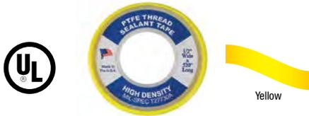
**YELLOW GAS LINE PTFE TAPE** 4 mil thick, 0.9g/cm<sup>3</sup> high density. Specifically formulated for use on natural, LP and synthetic gases. UL Approved. Meets or exceeds MIL-T-27730A. Meets International Fuel Gas Code 403.9.3 for Thread Joint Compounds. **Made in the U.S.A.**
