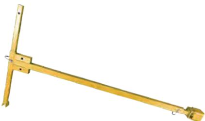
**FIBERGLASS SHAFT SOIL PROBES\*** With fiberglass "T" handle. 1/2" (1.27 cm) diameter shaft has heavy duty zinc metal tip for durability and ease of extraction. Safe, nonconductive probe for locating irrigation, power and water lines. Probes are constructed of solid yellow fiberglass that will not weather, warp or splinter. **Made in the U.S.A.**
