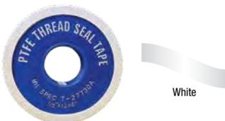
**QUALITY WHITE MEDIUM DENSITY PTFE TAPE** Pipe joint compound in tape form. Packed on a spool with cover. 3.5 mil thick, 0.38g/cm<sup>3</sup> density. Meets MIL-T-27730A. Meets International Fuel Gas Code 403.9.3 for Thread Joint Compounds.
