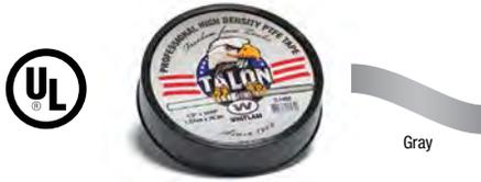
**TALON PROFESSIONAL HIGH DENSITY GRAY PTFE TAPE** 3.5 Mil Thick, 0.8g/cm<sup>3</sup> high density, 100% elongation. Excellent for natural and LP gas. Meets MIL-T-27730A. Meets International Fuel Gas Code 403.9.3 for Thread Joint Compounds. Packaged in a point of purchase display box.
