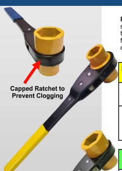
PLUMB-PRO® BoltTyte™ Through the Bolt Dual Socket Wrenches are professional grade two in one tools for gas and water industry couplings. Designed to be used on mechanical joints, flange bolts, repair clamps, service saddles, flange bolts, and sleeves. Excellent for mechanical joints/restraints, friction clamps, hydrant break flanges and most bonnet bolts.
