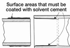
10. Apply cement lightly, but uniformly, to the inside of the fitting socket, taking care to keep excess cement out of the socket. This is to prevent solvent damage to the pipe. Time is important at this stage.
