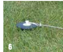
6 Attach string to lining peg and extend to next point. Now you can paint lines. Remove lining peg and string upon completion.
