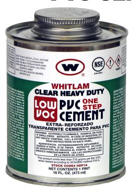
This solvent cement is suitable to be used as a One-Step Cement for joining PVC Drain, Waste and Vent (DWV) pipe and fittings in non-pressure applications in sizes up to and including 4 inches where acceptable by local code.
